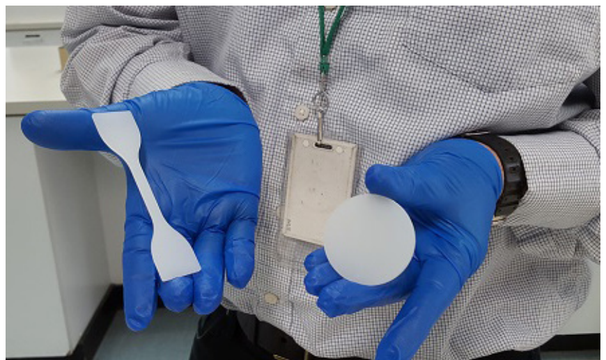
Samples exposed and tested in accordance with ASTM D543 at 23°C
