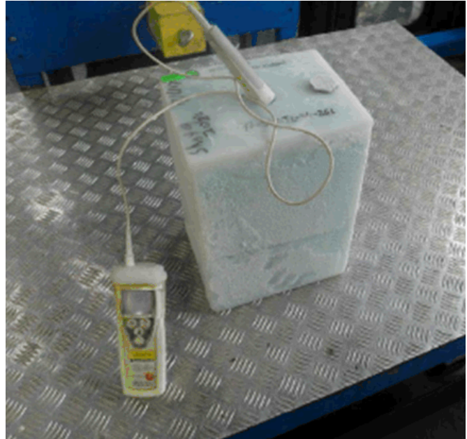
Alkatuff LL711UV undergoing low temperature impact testing
