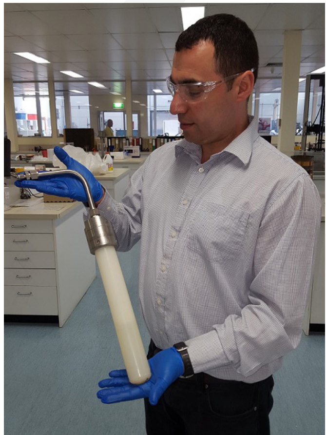
Rotational moulded pipe containing diesel fuel for storage testing
